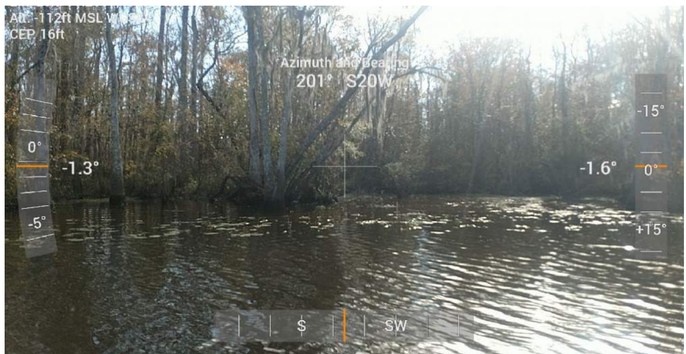
Figure 28: Chinquapin Canal, Cross Section 16041.2 looking at left overbank. The left overbank Manning's N value is estimated to be 0.11.
